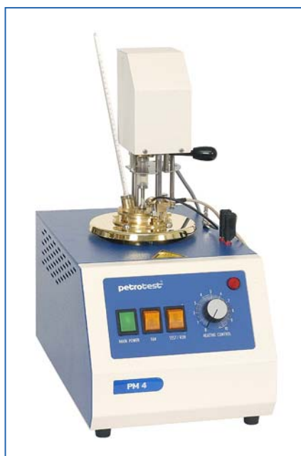
Fig 1. Petrotest PM4: Pensky-Martens Flash Point Tester with electric stirring and heating, gas + electric igniter and quick-connection head. Methods: ASTM D 93 A+B - IP 34 - DIN (EN) 22719 - ISO*2719 - NF M 07-019 - JIS K 2265
