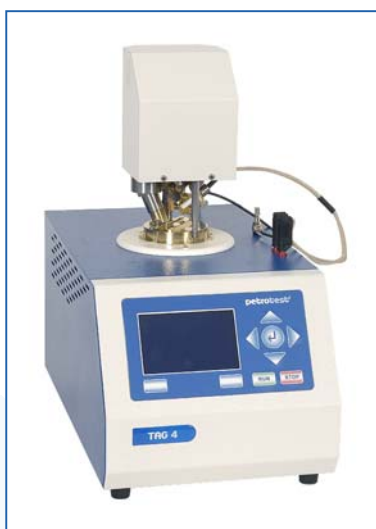
Fig 3. Petrotest TAG 4: Automatic TAG Closed Cup Flash and Fire Point Tester Suitable for fuels and diesel, featuring an automatic barometric pressure correction and safety shut off. Methods: ASTM D 56 - IP 304
