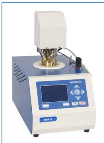
Fig 4. Petrottest ABA 4: Automatic Abel Flash Point Tester featuring Peltier elements for flash point measurements down to -20°C. Methods: IP 170 - IP 304 - ISO°1523 - NF M 07-011 - NF T 06-009
