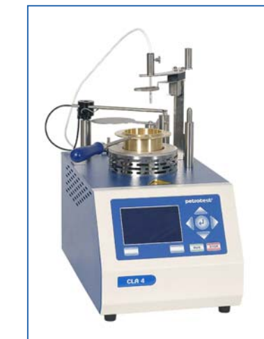
Fig 2. Petrotest CLA 4: Automatic Cleveland Open Cup Flash and Fire Point Tester. Suitable for oils and bitumens, featuring an automatically moveable test flame. Methods: ASTM D 92 - IP 36 - ISO 2592
