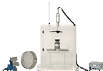
Herbert Corrosion Test Assembly
